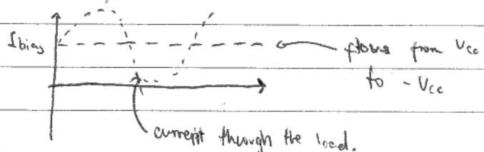
$\therefore$  Conduction angle =  $360^\circ$ .
