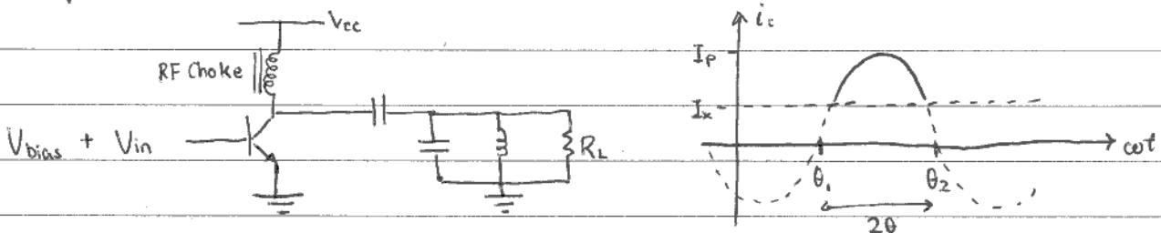
Usually used in RF transmitters operating at a single frequency where distortion is controlled by a tuned load.
