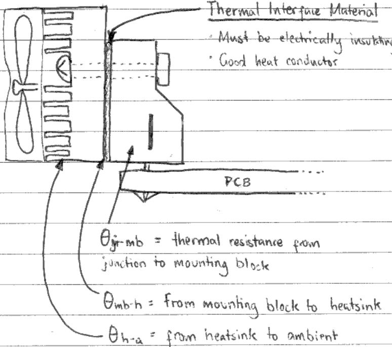
Heat sinks also have a large thermal capacity, modelled by C.
