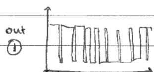
The low-pass filtered signal is an amplified replica of the input.
